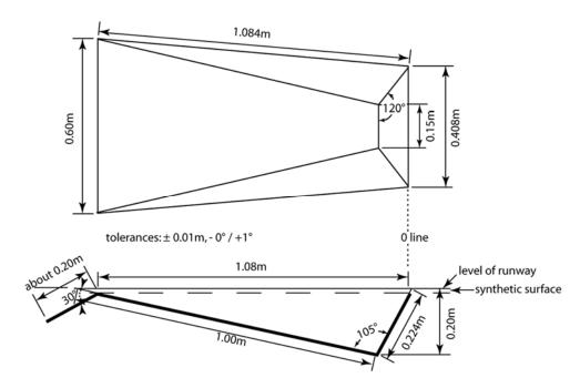
Figure (a) TR28 (Rule 183) - Pole Vault box (top and side view)
