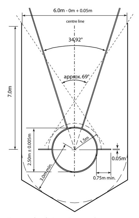
Figure TR35 (Rule 190) - Cage for Discus Throw only (with cage dimensions to netting)
