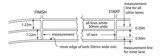
Figure TR14 (Rule 160) - Track measurements (infield view)
