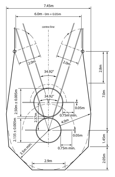
Figure (c) TR37 (Rule 192) - Cage for Hammer and Discus Throw with separate circles
