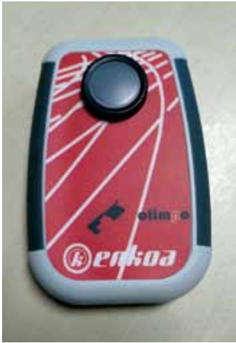
Figure 6: Olimpo Device Coach's Remote Control Unit
