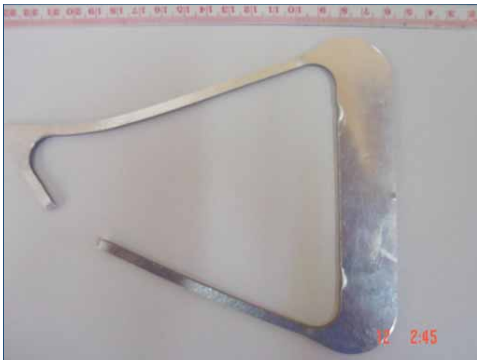
Figure 11: ADFA-1 Hammer handle after failure
