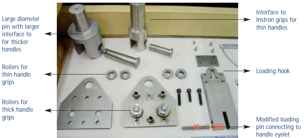
Figure 3: Components of a modified test fixture
