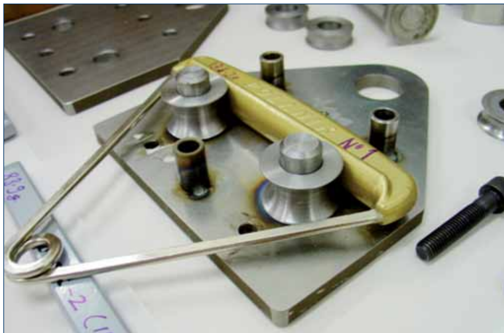
Figure 4: Handle in the modified test fixture (Note: the thick ridge along the base of the grip)
