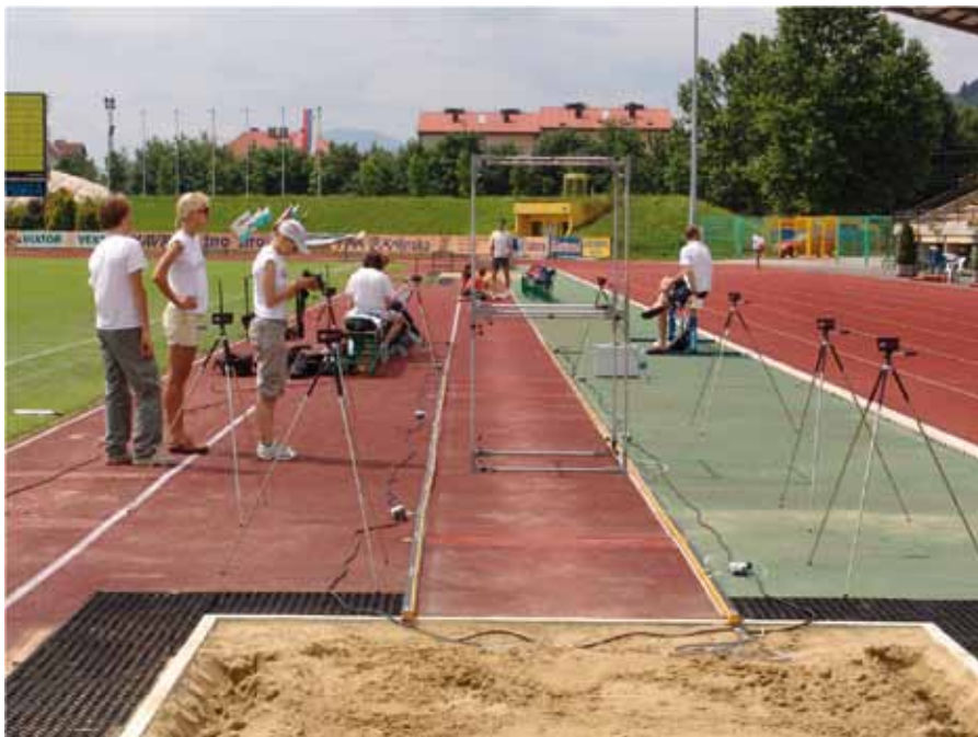
Figure 3: Calibration – the procedure for comparing spatial measurements from different devices
